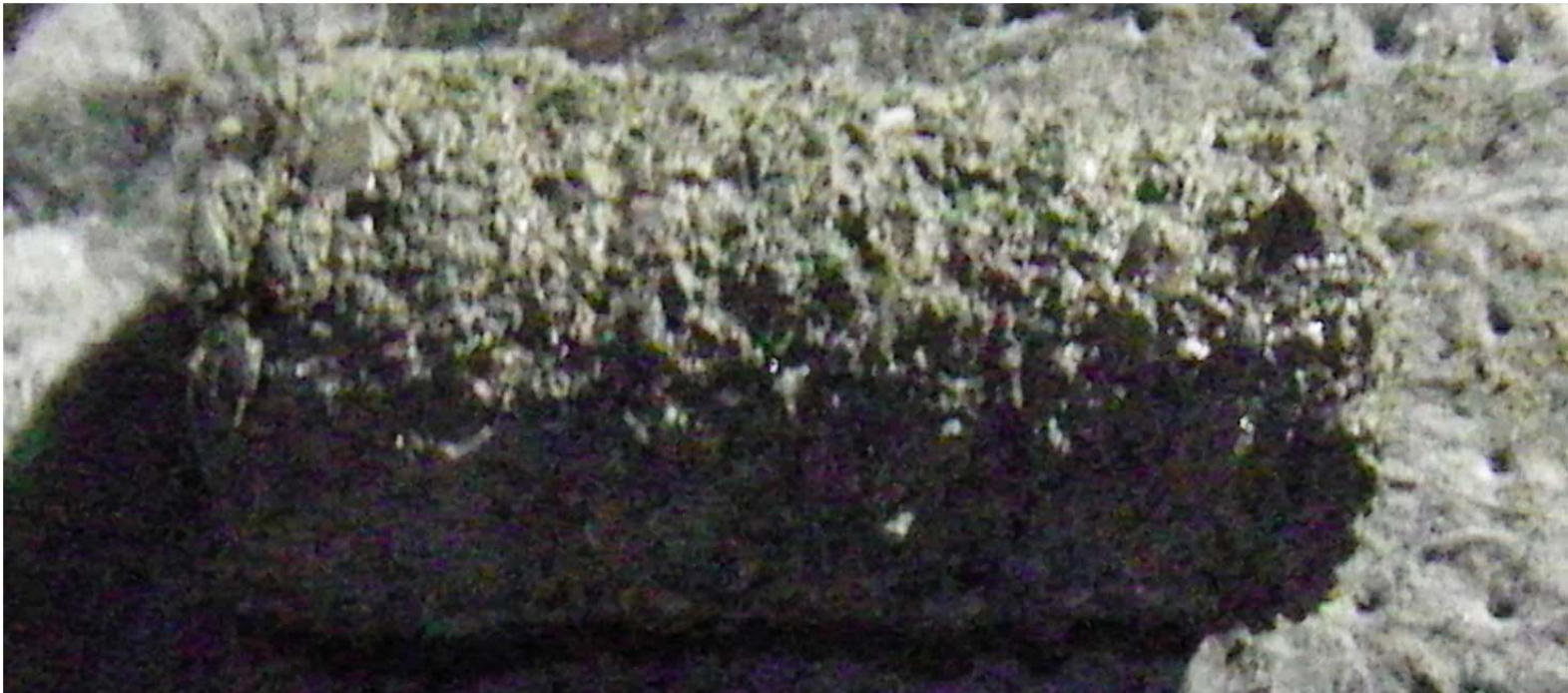
Photo 14: Drilled core HB12-ND-CORE-DC12-QA-20120130 collected from station 0+55 downstream. This core is of the lift placed 2012/01/29 nightshift.
